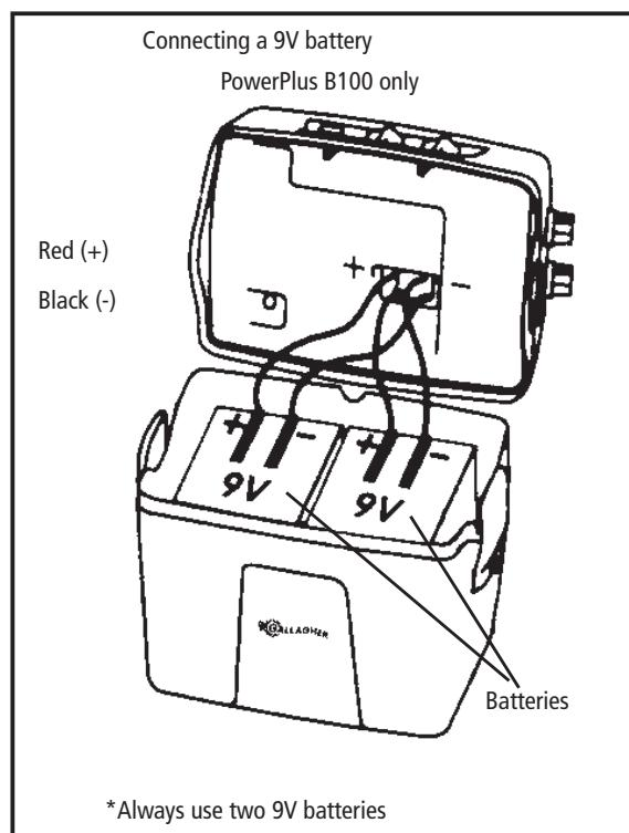
ALWAYS leave battery (batteries) disconnected during storage.
